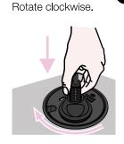
LOCKING POSITION **E** LOCKING POSITION Rotate clockwise.
