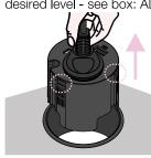
Note! Pay attention to the locking geometry as it will help with adjusting the inner part to the desired level.
