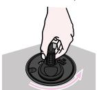
ADJUSTING HEIGHT The inner part should now be loose. Adjust to desired level - see box: ADJUST LEVELS
